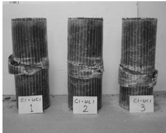
**Figure 4. Failure of C1-UC1**
