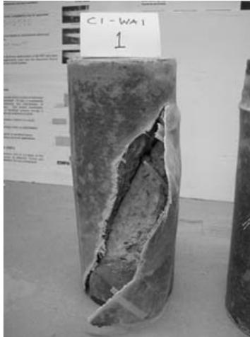
**Figure 12. Global Concrete Shear Crack**
