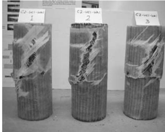
**Figure 6. Failure of C2-UC1-WA1**
