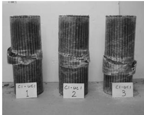
**Figure 4. Failure of C1-UC1**
