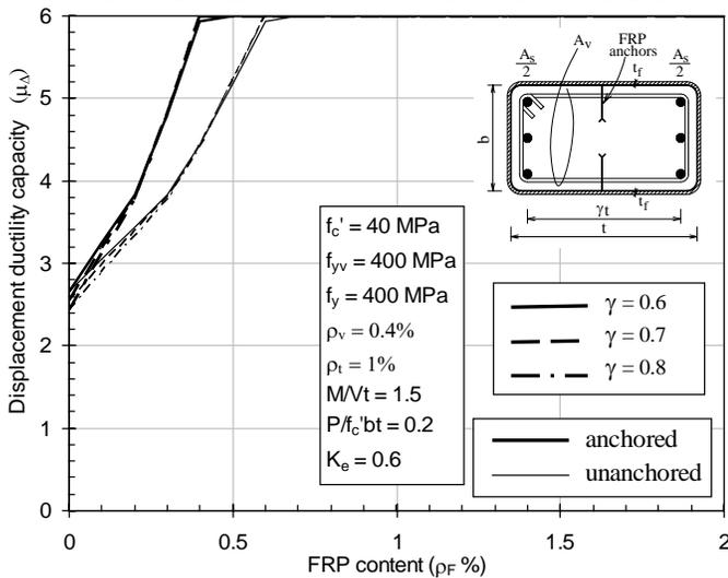
Figure 6. Effect of the ratio of the distance between longitudinal reinforcement-to-the overall depth on the  $\mu_{\Delta}$ - $\rho_F$  relationship.
