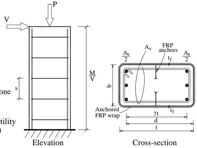
Figure 2. FRP-rehabilitated rectangular RC subjected to lateral displacement.
