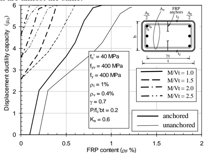
Figure 7. Effect of shear span-to-depth ratio on the  $\mu_{\Delta}$ - $\rho_F$  relationship.
