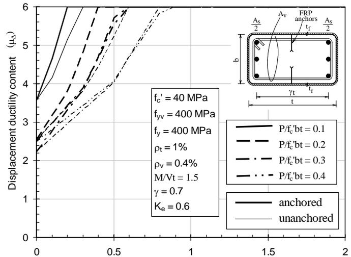
Figure 12. Effect of axial load on the  $\mu_\Delta$ - $\rho_F$  relationship.
