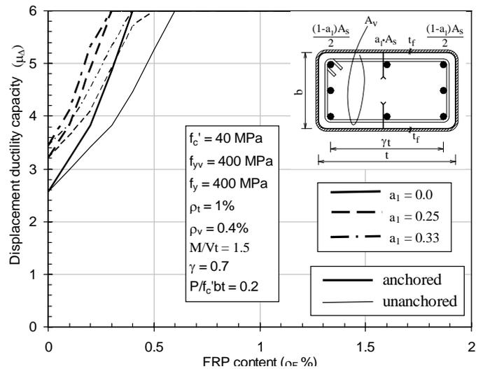
Figure 11. Effect of the longitudinal bar arrangement on the  $\mu_\Delta$ - $\rho_F$  relationship.
