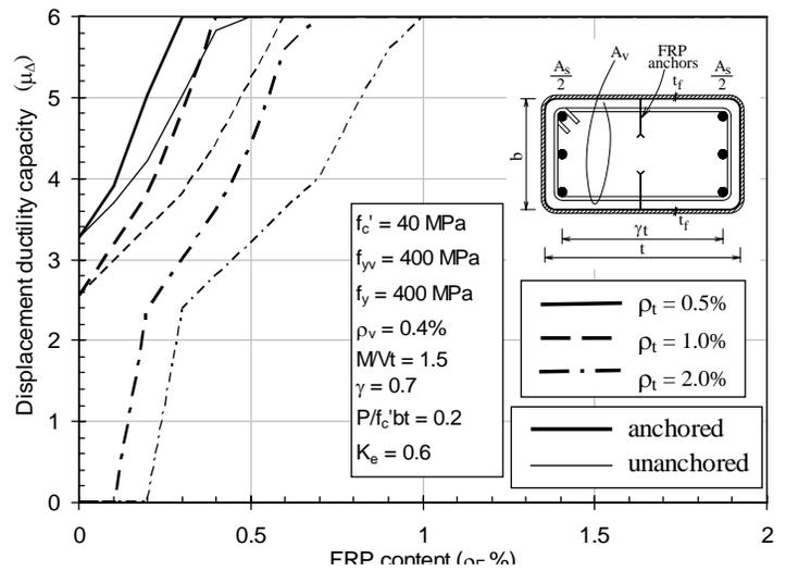
Figure 9. Effect of longitudinal reinforcement content on the  $\mu_{\Delta}$ - $\rho_F$  relationship.
