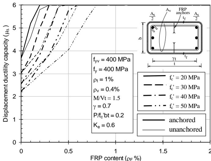
Figure 3. Effect of the concrete compressive strength on the  $\mu_\Delta$ - $\rho_F$  relationship.
