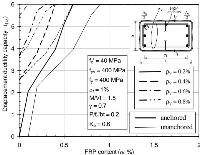
Figure 8. Effect of transverse reinforcement content on the  $\mu_{\Delta}$ - $\rho_F$  relationship.
