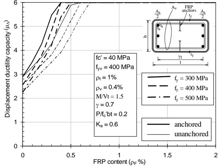
Figure 5. Effect of the yielding strength of longitudinal reinforcement on the  $\mu_{\Delta}$ - $\rho_F$  relationship.
