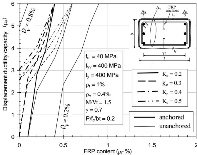
Figure 10. Effect of the confinement coefficient  $K_e$  on the  $\mu_\Delta$ - $\rho_F$  relationship.
