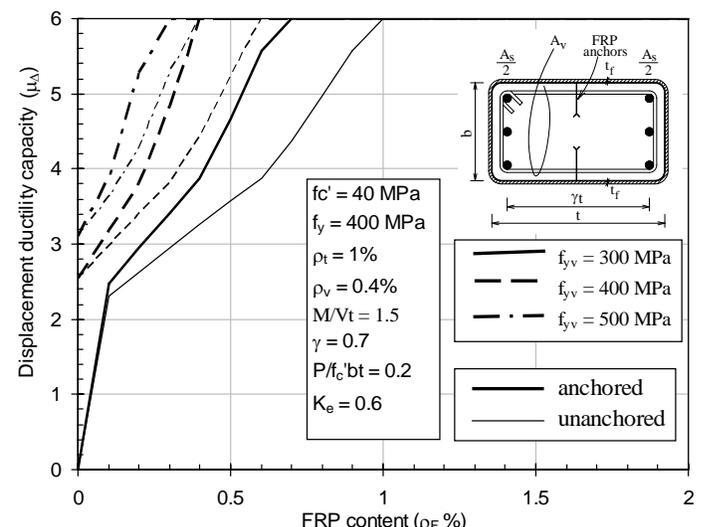
Figure 4. Effect of the yielding strength of transverse reinforcement on the  $\mu_\Delta$ - $\rho_F$  relationship.
