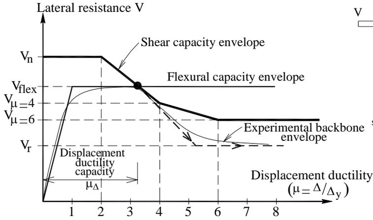
Figure 1. Shear capacity-displacement ductility model for FRP-rehabilitated columns (Galal et al. 2005).
