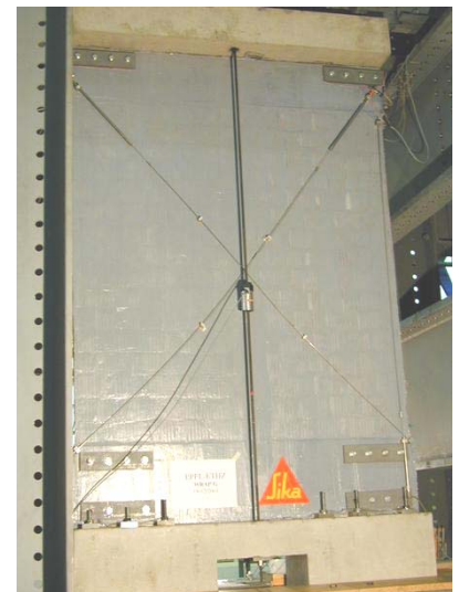
Figure 7. Wall Specimen WRAP-G Upgraded On One Side (West Side) Using GFRP.
