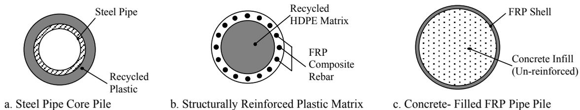
**Figure 2.** Some Common Types of Composite Piles
