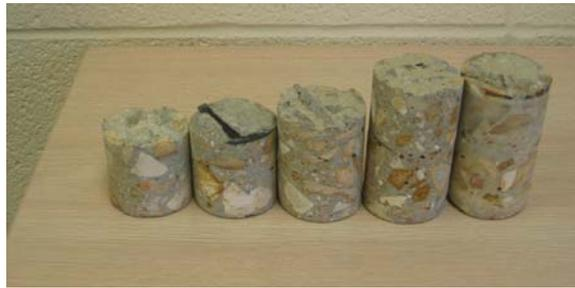
**Figure 18. Disbond between substrates**
