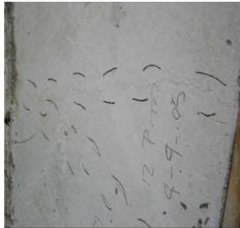
d) Transversal Crack in Control Slab
