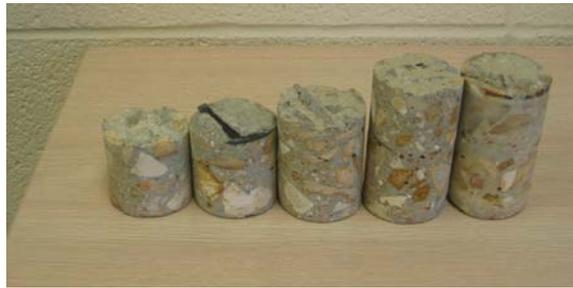
**Figure 18. Disbond between substrates**
