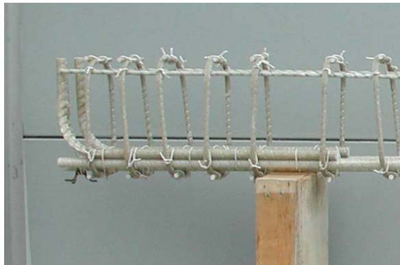
(a) Lap Splice at Bar Ends
