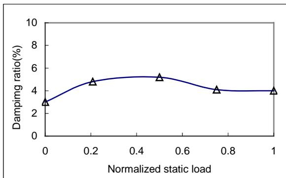
**Figure 5.9** Change of damping with static load
