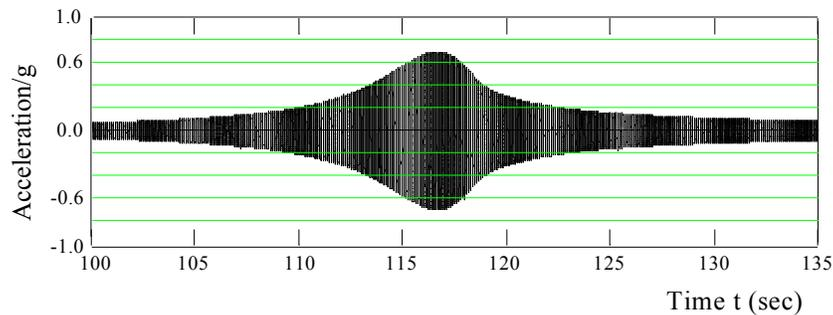
**Figure 6.2** Analytical response at midspan of beam under swept-sine loading
