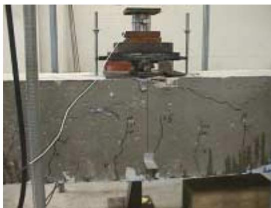
**Figure 4.16** Failure of a CFRP strengthened beam
