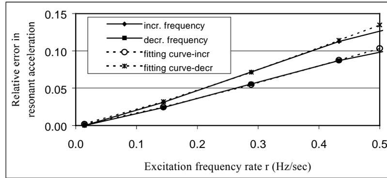
**Figure 6.6** Effect of excitation frequency rate on resonant acceleration at midspan
