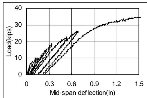
**Figure 4.3** Load versus midspan deflection of Beam 3
