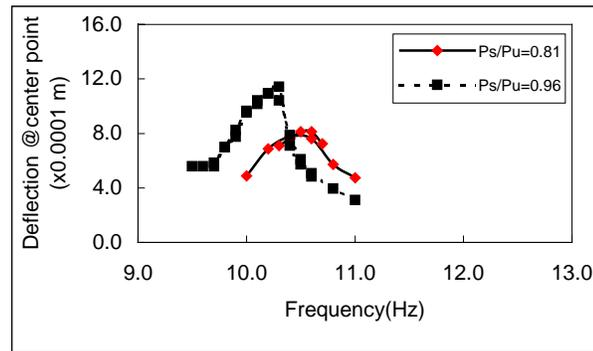
(b)  $W_p/W_{beam}=0.3$ **Figure 4.9** Preload effect on transfer function
