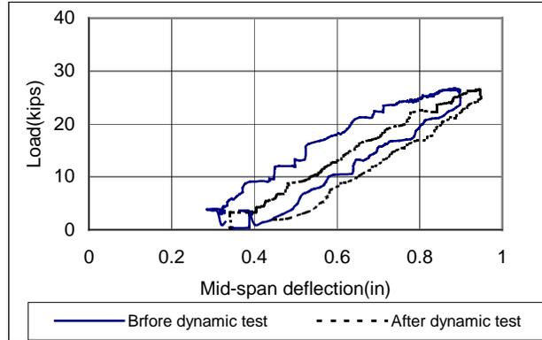
**Figure 4.5** Dynamic effect on beam responses ( $P_s=26$  kips)
