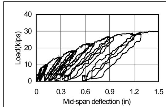
**Figure 4.1** Load versus midspan deflection of Beam 1
