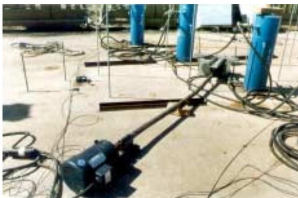
**Figure 5.3** Static and dynamic loading system
