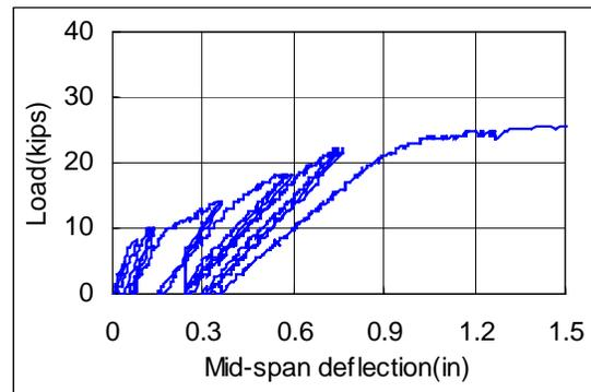
**Figure 4.2** Load versus midspan deflection of Beam 2
