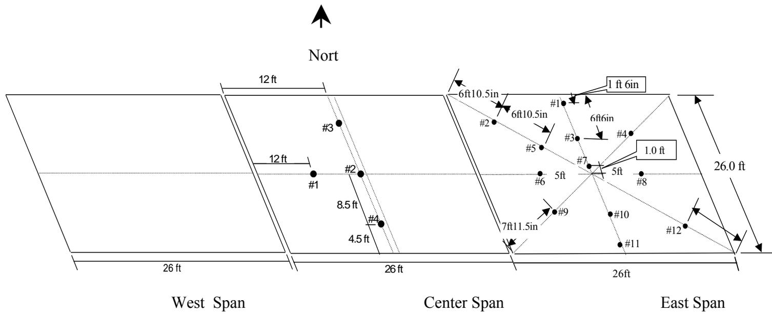
**Figure 5.2** Location of accelerometers
