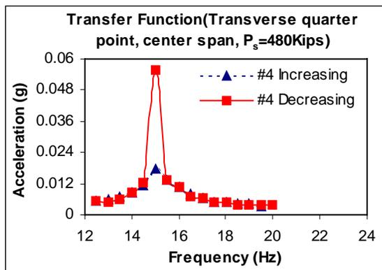
**APPENDIX E:****TRANSFER FUNCTIONS OF BEAM 2 FROM SWEPT-SINE TESTS**
