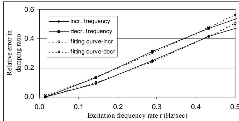
**Figure 6.7** Effect of excitation frequency rate on damping ratio
