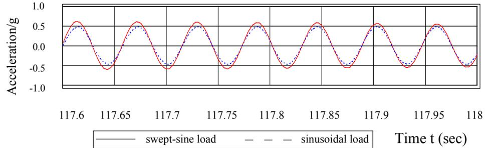
**Figure 6.3** Response comparison under swept-sine and sinusoidal loads
