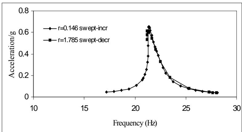
**APPENDIX F:****TRANSFER FUNCTIONS OF BEAM 3 FROM SWEPT-SINE TESTS**
