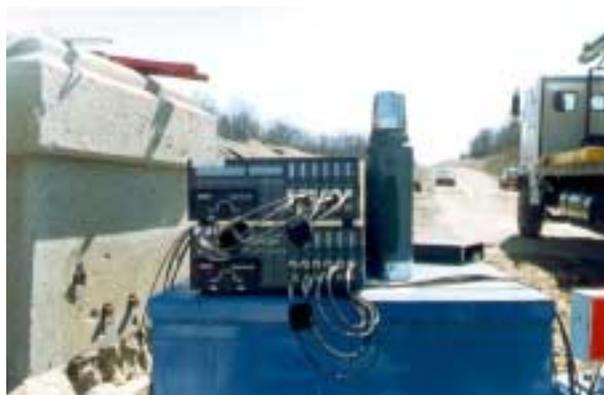
**Figure 5.5** Data acquisition system
