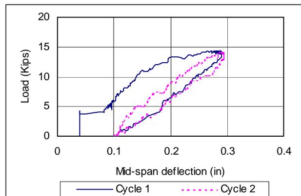
**Figure 4.4** Stiffness degradation of Beam 1 ( $P_s=14$  kips)
