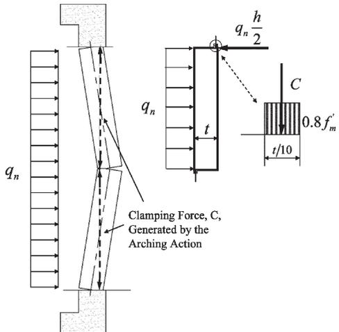
Figure 4 – Design of Rigid Arching Walls
