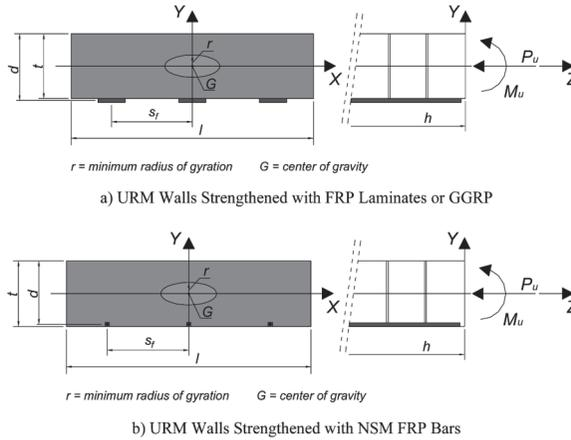
Figure 2 — Geometric parameters of the uncracked section under out-of-plane loads with axial compression
