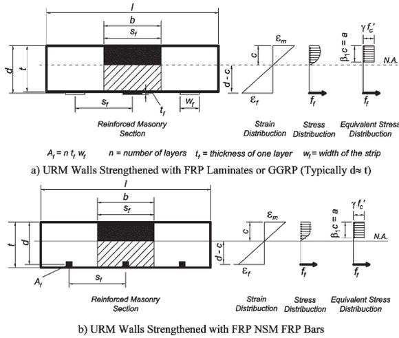
Figure 1 — Internal strain and stress distribution for a horizontal rectangular section of a strip of masonry under out-of-plane loads, without axial compression
