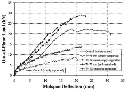
Figure 3 – Comparison between Simply Supported and End-Restrained Walls
