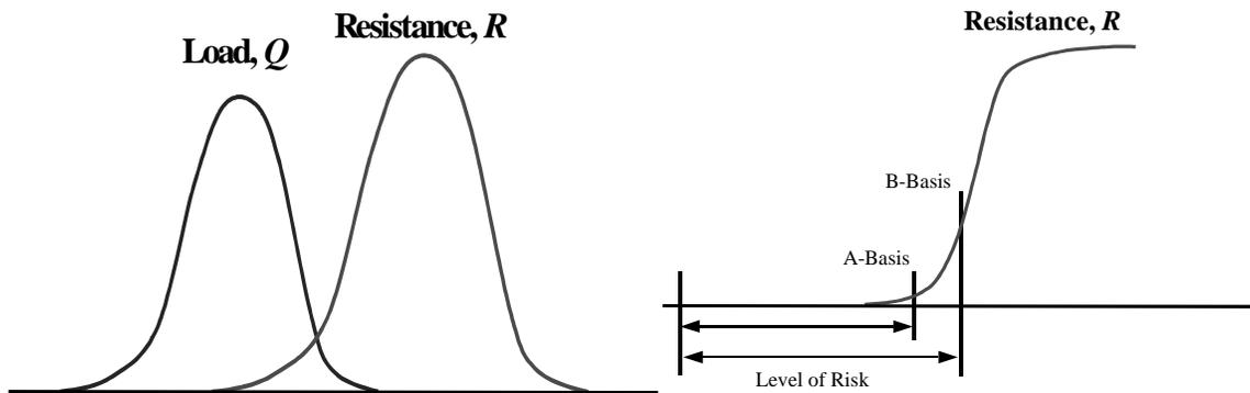
**Figure 2.** LRFD conceptual representation for design; A- and B-Basis Allowables
