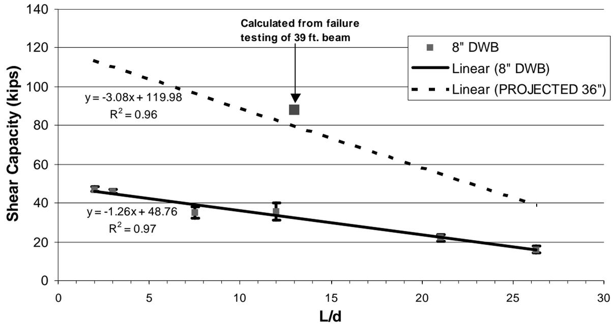
**Figure 4.** Shear capacity vs. L/d for 8-inch DWB and *initial* prediction for the 36-inch DWB
