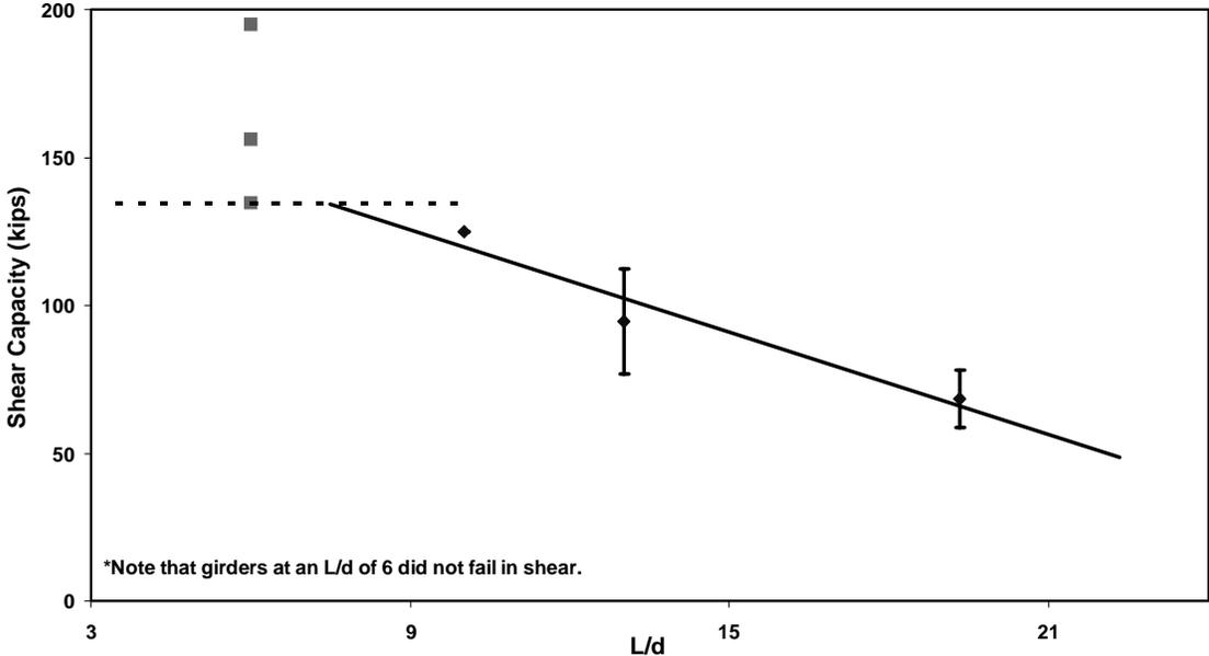
Figure 8. Average Shear Capacity versus L/d, 36-inch DWB, Error bars represent one standard deviation; Data points at L/d of 6 were bearing failures
