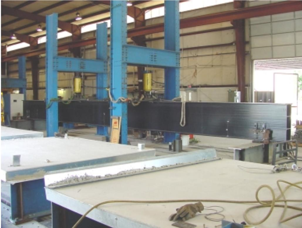
**Figure 5.** Four-point bending test setup of 36-inch DWB
