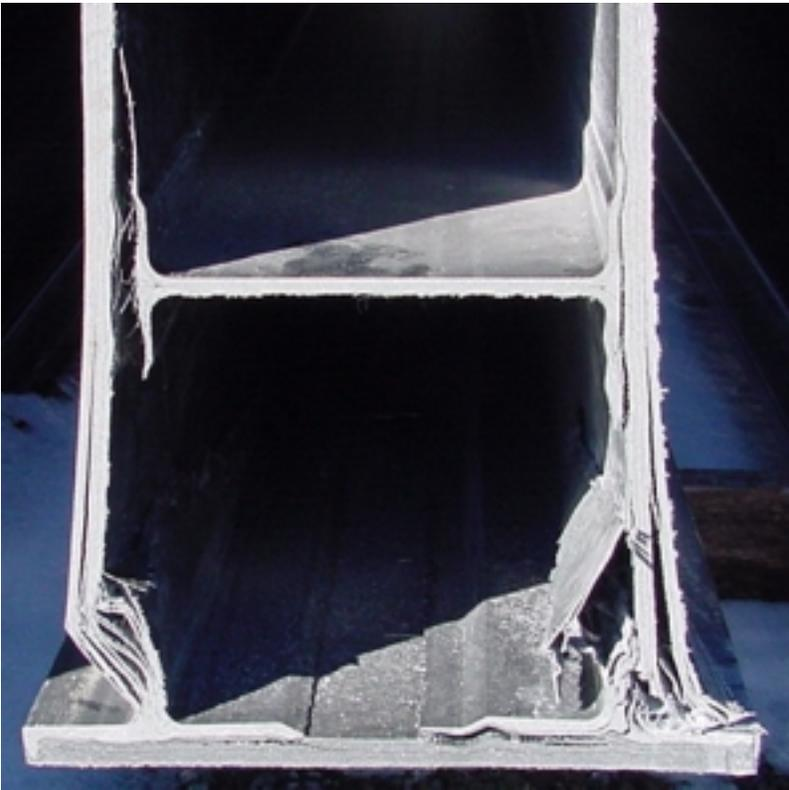
Figure 7. Bearing Failure of 36-inch DWB, 20-ft span
