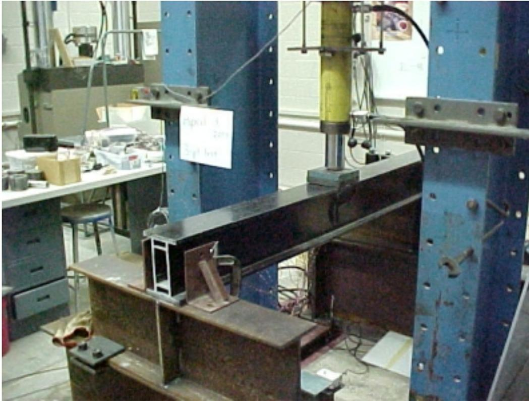
**Figure 3.** Short span three-point bending test setup
