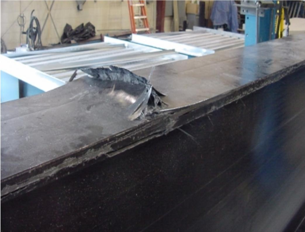
**Figure 6.** Delamination of the compressive flange of a 36-inch DWB near a loading patch.
