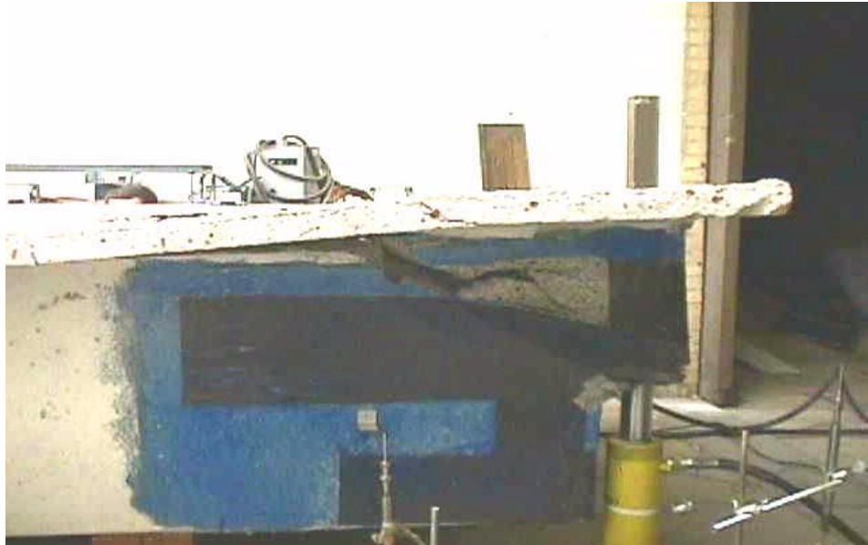
Figure H.3: Inclined Cracks at the Reentrant Corner Extended to the Web-Flange Junction of Specimen 1F-8
