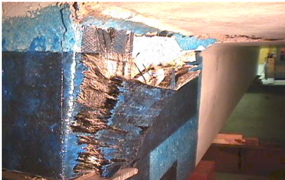
Figure H.4: Failure of Dapped-end Due to the Peeling of FRP Laminates in Specimen 1F-8
