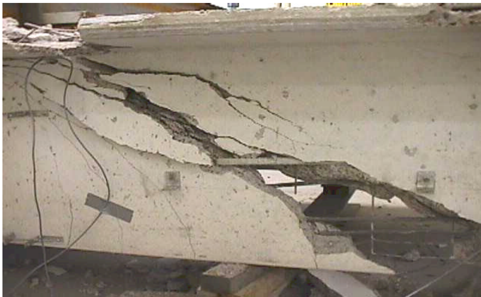
Figure H.6: Crushing of Concrete in the Interface of Shear-Flexure Crack in Specimen 1S-8
