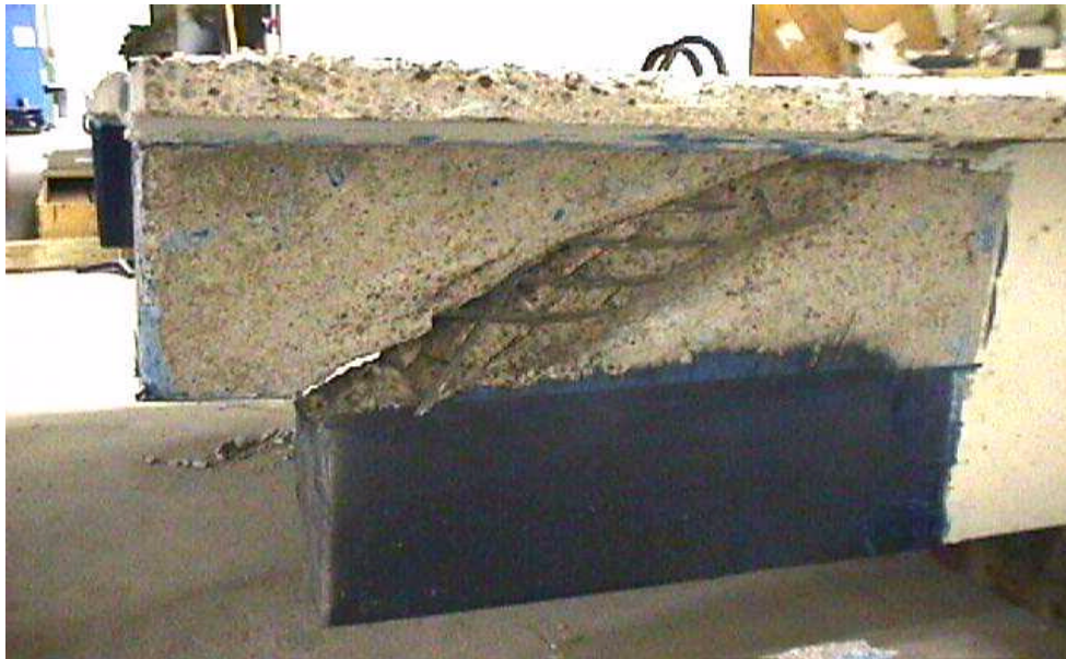
Figure H.11: 45° Crack from the Reentrant Corner Caused the Failure of Specimen 3F-5
