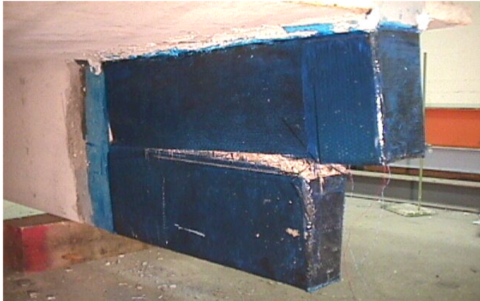
Figure H.9: Shear Failure of Dapped-end at the Reentrant Corner Due to the Fiber Rupture in Specimen 3F-5
