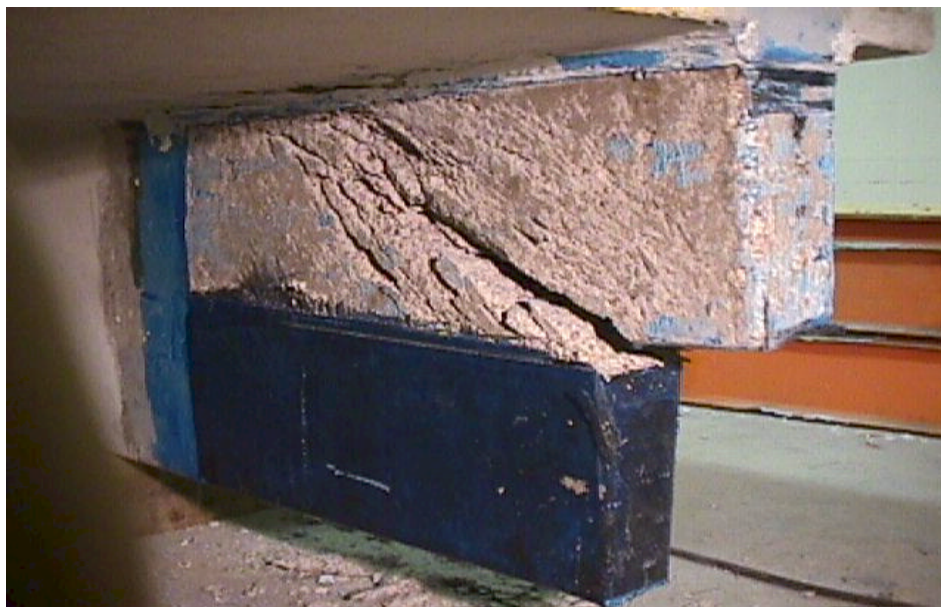
Figure H.10: 45° Crack from the Reentrant Corner Caused the Failure of Specimen 3F-5
