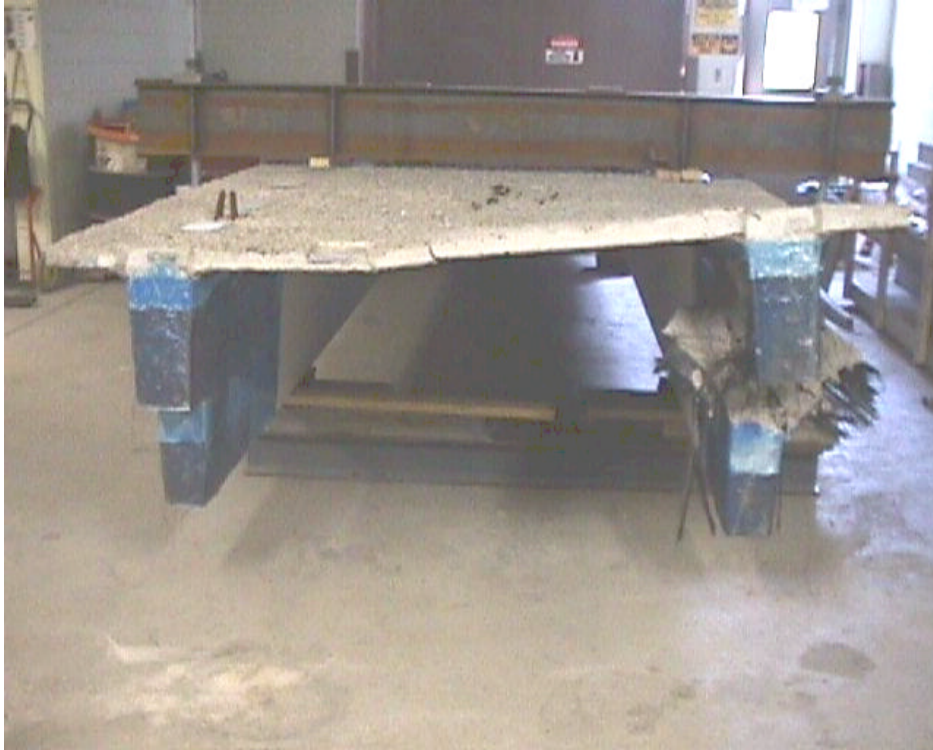
Figure H.7: Failure of Dapped-end Due to the Peeling of FRP Sheets at the Reentrant Corner of Specimen 2F-8
