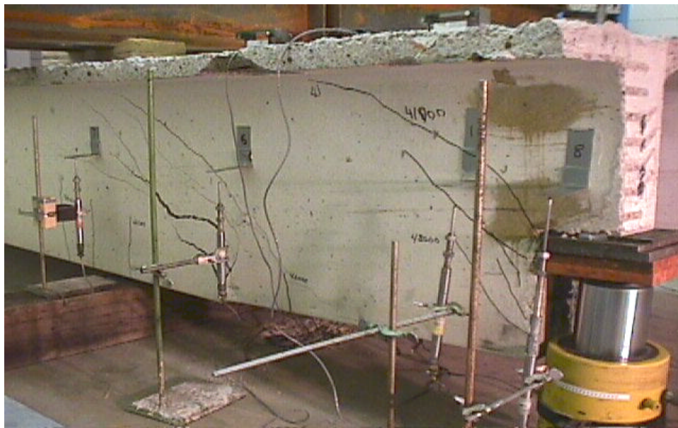
Figure H.12: Shear-flexure Failure in West Stem of Specimen 3S-5
