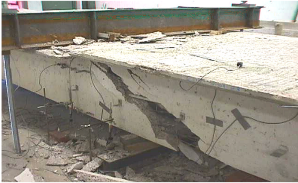
Figure H.5: Failure of Steel Reinforced Specimen Due to the Shear-flexure Crack Extended to Top Support of Specimen 1S-8
