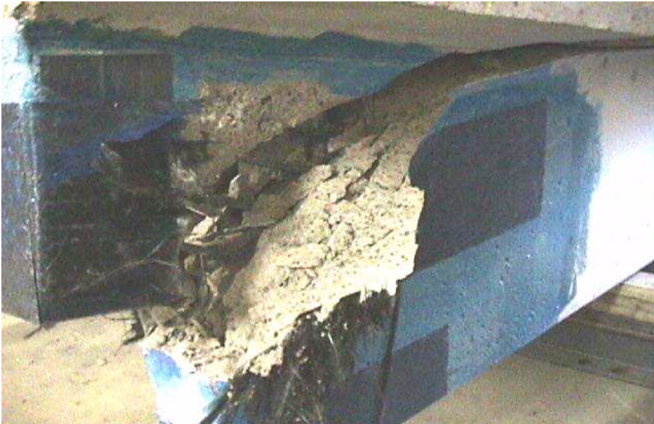
Figure H.8: Close Look of Shear Failure at the Reentrant Corner of Specimen 2F-8
