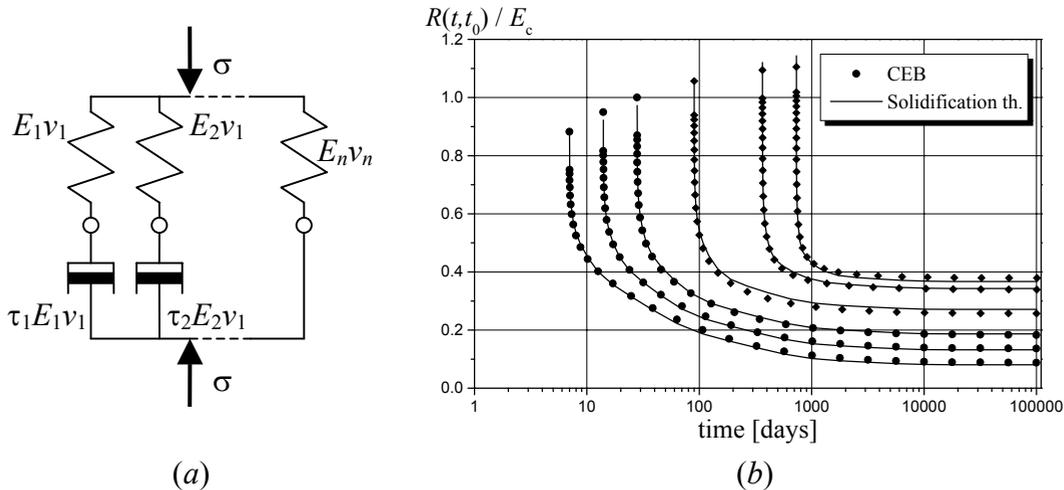
**Figure 2:** (a) Maxwell chain composed of  $N$  units; (b) best fitting of CEB relaxation curves using solidification theory (RH%=50,  $f_{cm}$ =38 Mpa,  $2A_c/u$ =50 mm).
