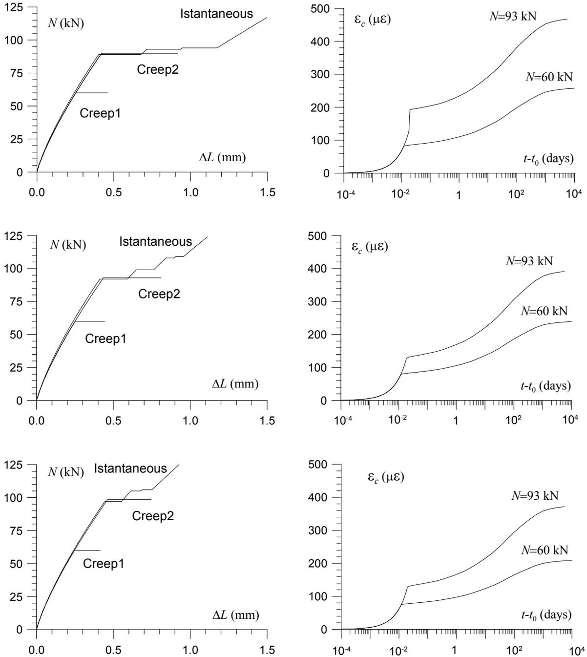
**Figure 4:** Instantaneous and long term force-elongation diagrams and strain evolution with time. (a, b) unplated, (c, d)  $h_p=0.33$  mm; (e, f)  $h_p=1.016$  mm.
