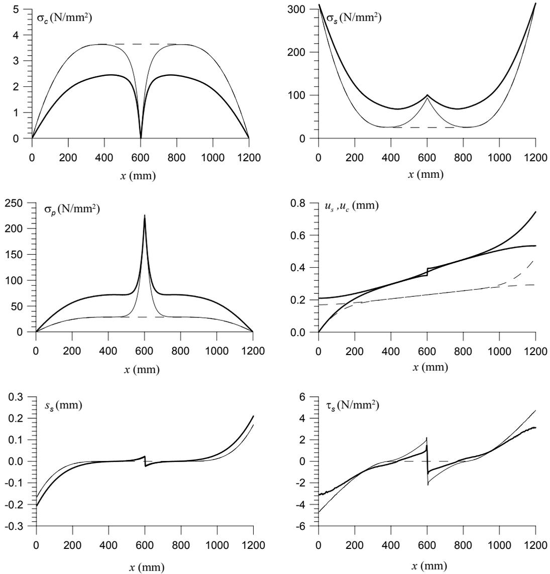
**Figure 5:** FRP-reinforced tensile member ( $h_p=1.016$  mm): (a) concrete stress; (b) steel stress; (c) stress in FRP plates; (d) Steel and concrete displacements; (e) steel-concrete slip; (f) steel-concrete bond shear (---: before concrete crack; —: after crack; —: long time values: 30 years).
