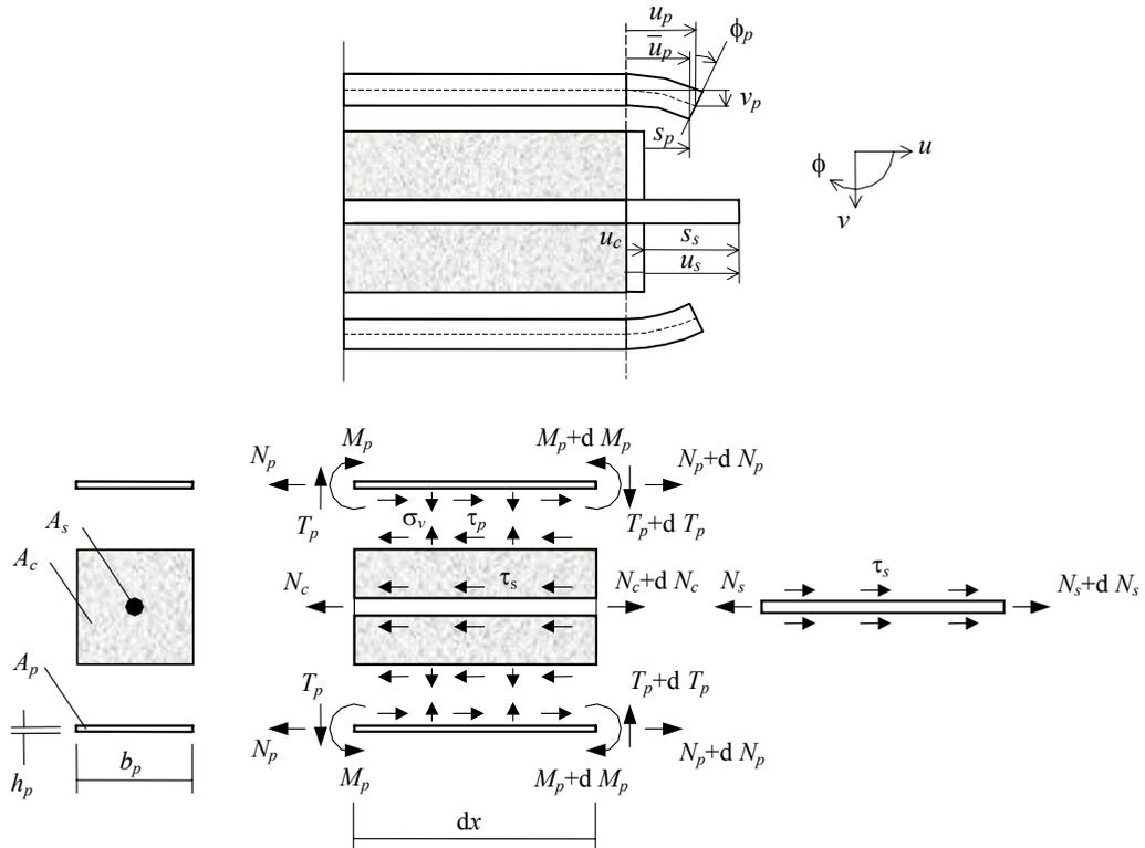
**Figure 1:** Notation adopted for displacements and forces for concrete, steel bars and plates.
