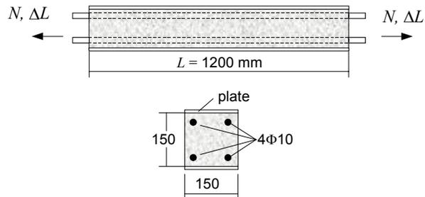
**Figure 3:** Geometry and mechanical properties of FRP-reinforced tensile member considered in numerical examples.
