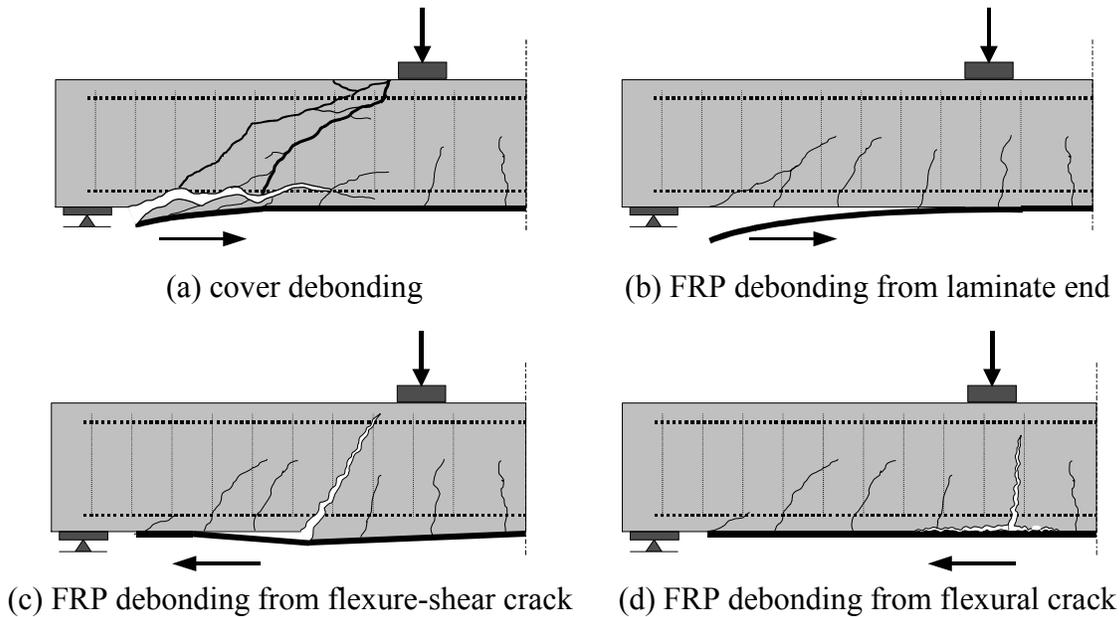
FIG 1. Debonding failure mechanisms
