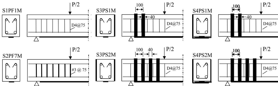
(b) beams strengthened in shear and/or flexure in various configurations
