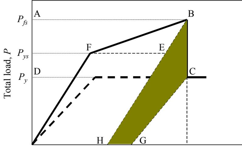
FIG. 4. Potential energy difference in the beam upon debonding failure
