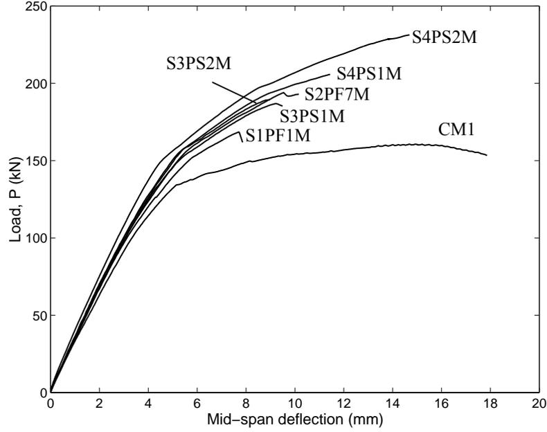
FIG. 3. Load-deflection curves of tested beams
