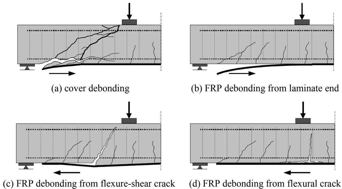
FIG 1. Debonding failure mechanisms
