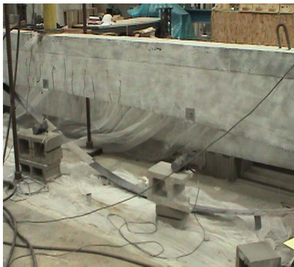
(c) Beam 4 after failure
