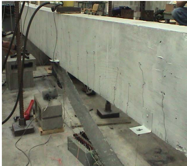
(a) Beam 3 after failure
