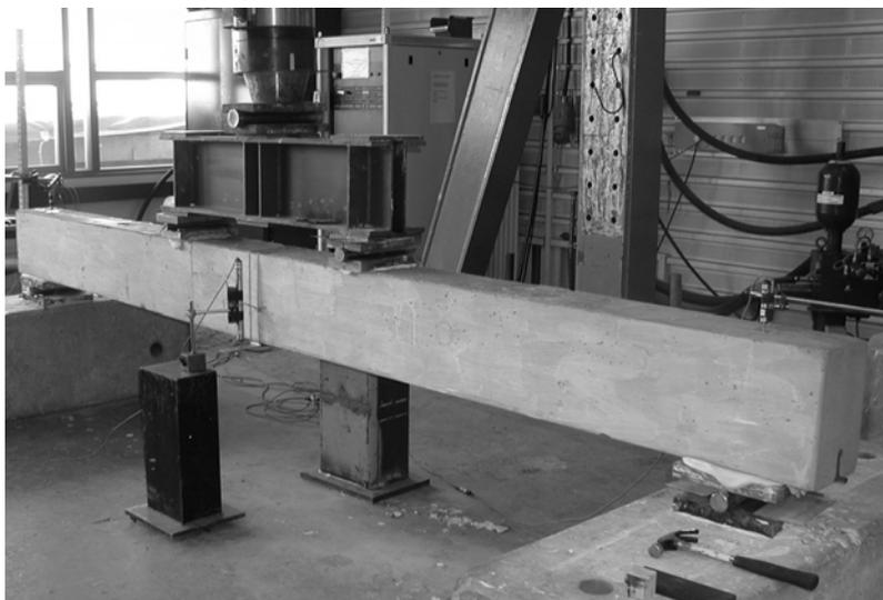
**Figure 7.** Beam setup during testing
