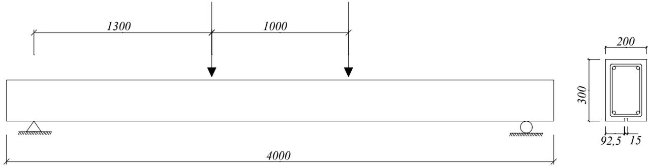
**Figure 4.** Beam test setup
