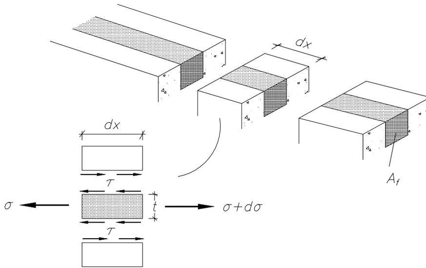
**Figure 3.** Shear stresses acting on a small element  $dx$  of NSMR rod
