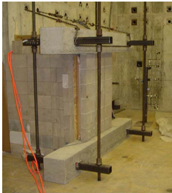
Figure 1. Test Set-Up for Static Load Tests (Control Wall)
