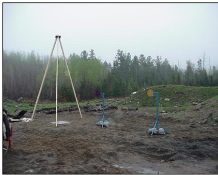
Fig. 4. The test specimen and the tripod holding the explosive charge.
