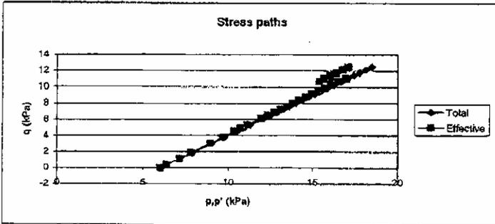
Undrained triaxial test (BV-1 TW5)
