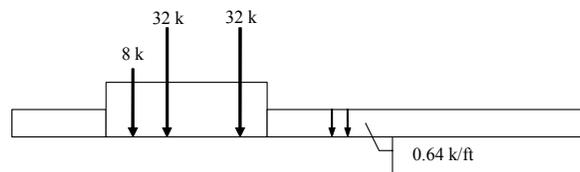
(b) Load Lane Representing a HS20 Truck Plus a Uniform Live Load
