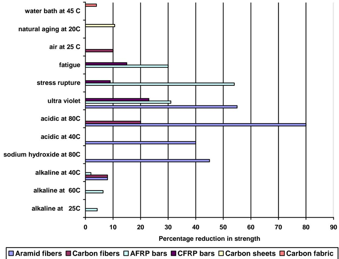
**Figure 3. Strength Degradation of FRP material alone**
