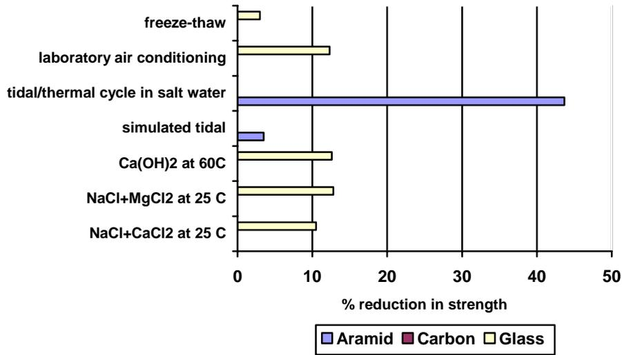
**Figure 1. Strength Degradation in Internally bonded FRP**
