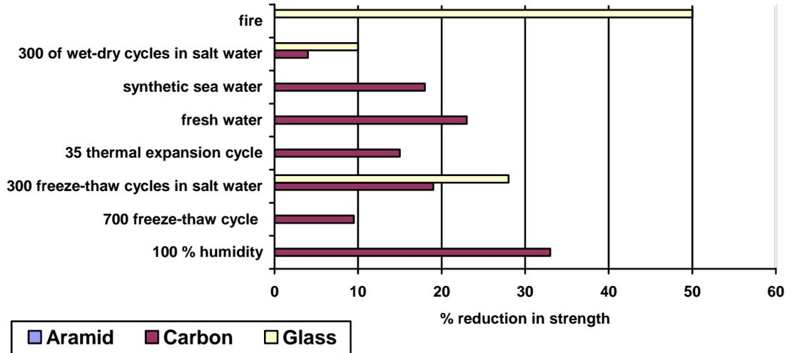
**Figure 2. Strength Degradation in Externally bonded FRP**
