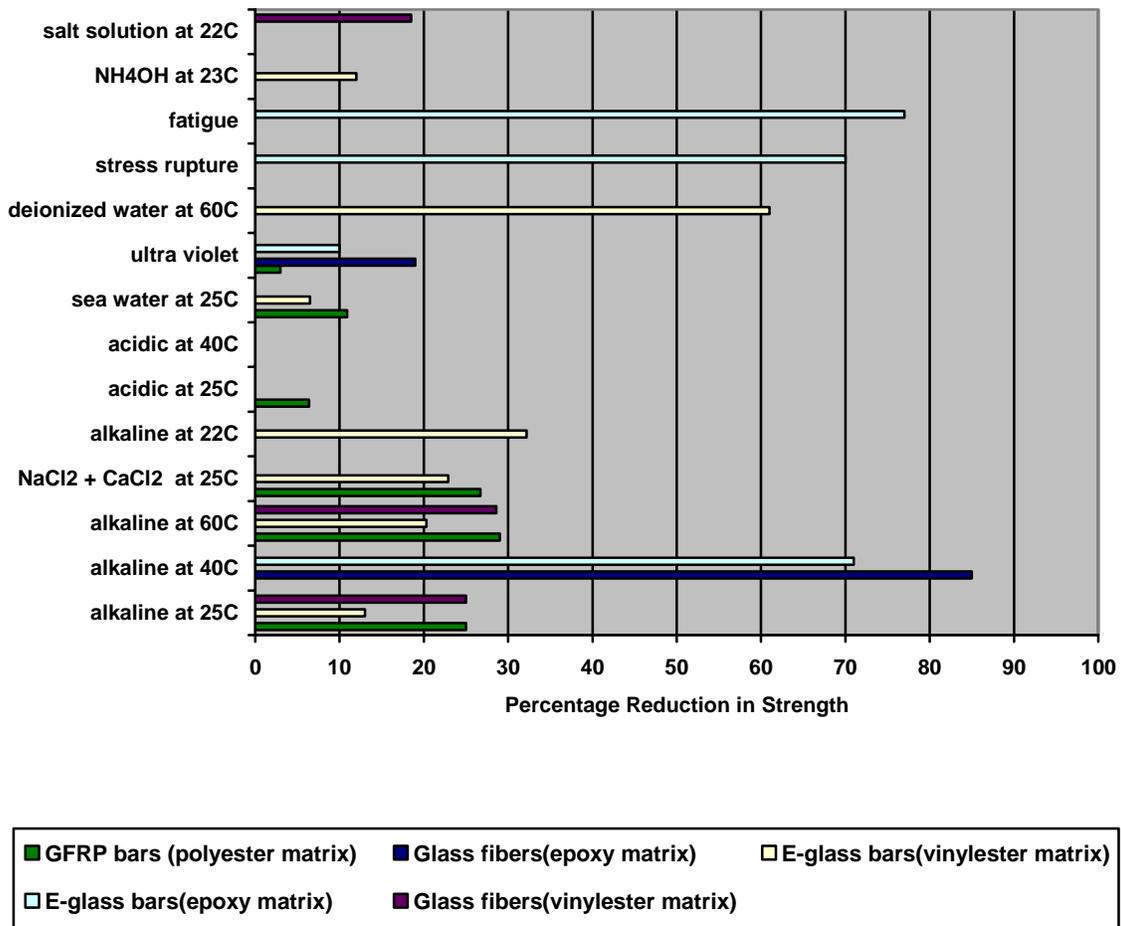
**Fig 4 Strength Degradation of Glass FRP alone**
