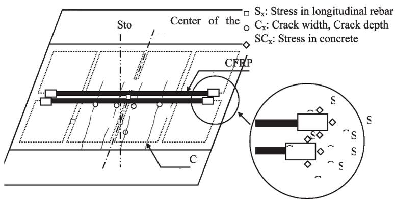
Figure 7—Measurement points of prestress introducing test
