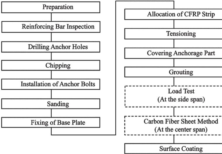
Figure 4—Application Procedure
