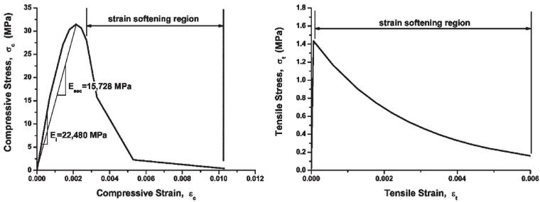
(a) Compressive stress-strain relationship      (b) Tensile stress-strain relationship
