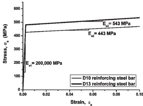
Figure 3 – Property of reinforcing bar
