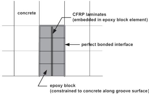
Figure 5 – Boundary conditions at interface
