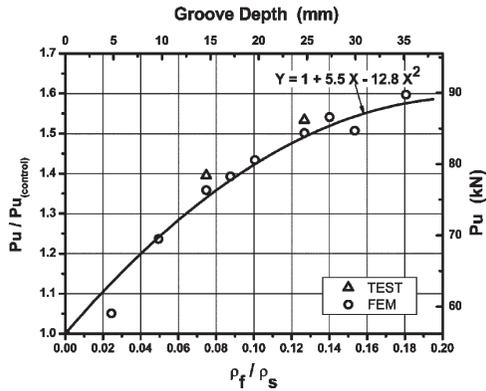
Figure 9 – Increase rate of ultimate load vs. reinforcement area ratio
