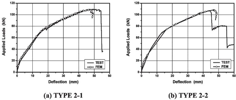
Figure 8 – Comparison of analytical and experimental results according to spacing
