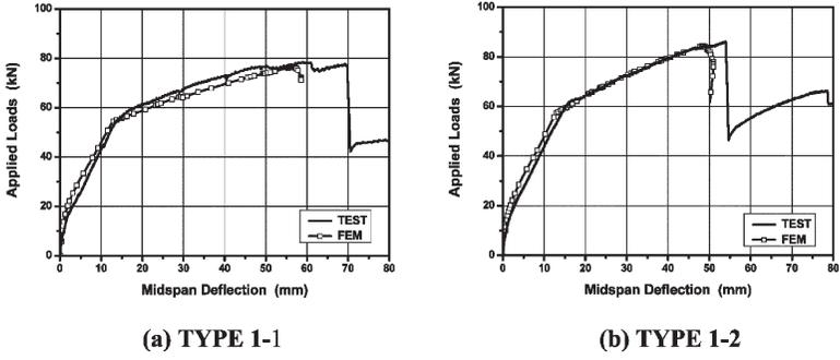
Figure 7 – Comparison of analytical and experimental results according to groove depth
