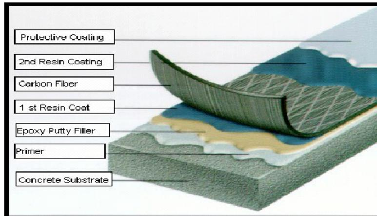
Figure 1 External Bonding with FRP Laminates
