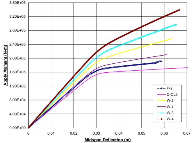
Figure 3 Load-Deformation of FRP-Strengthened RC Girders
