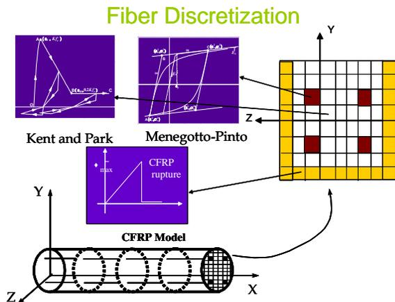
Figure 2 Modeling of FRP-Strengthened RC Girders
