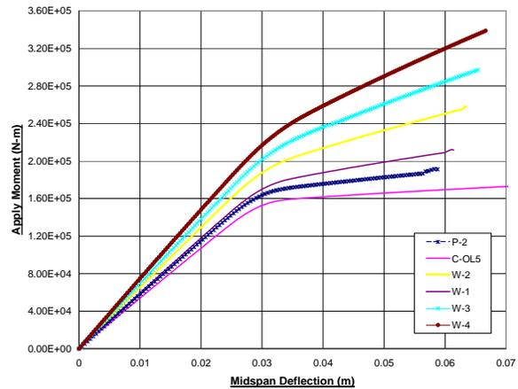
Figure 5 Load-Deformation Behavior of Shahawy Beams
