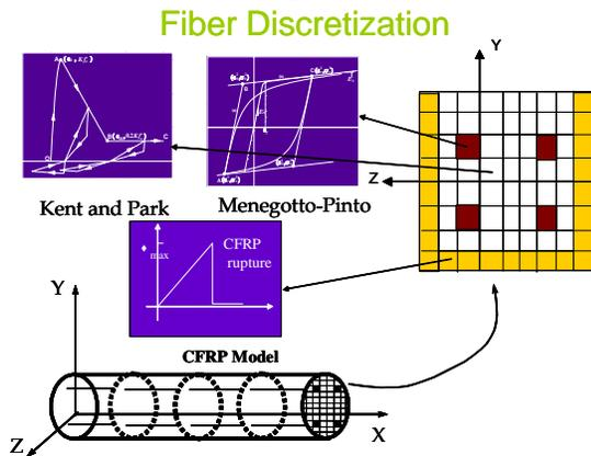
Figure 2 Modeling of CFRP-Strengthened RC Girders
