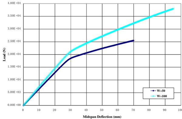
Figure 9 Load-Midspan Behavior of Zarnic Beam
