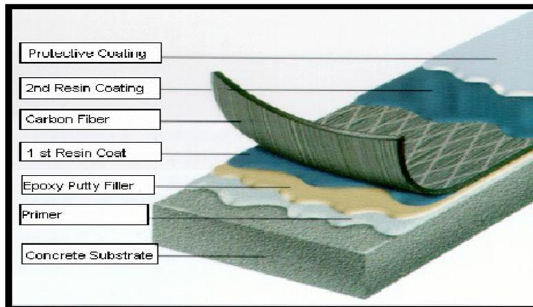
Figure 1 External Bonding with CFRP Laminates
