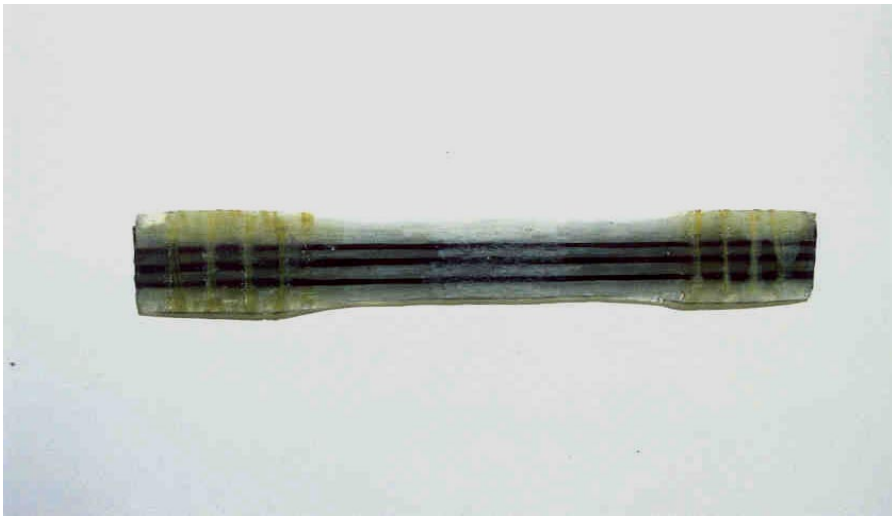
Figure 1. Test Sample for the Developed Uniaxial Hybrid Fabric
