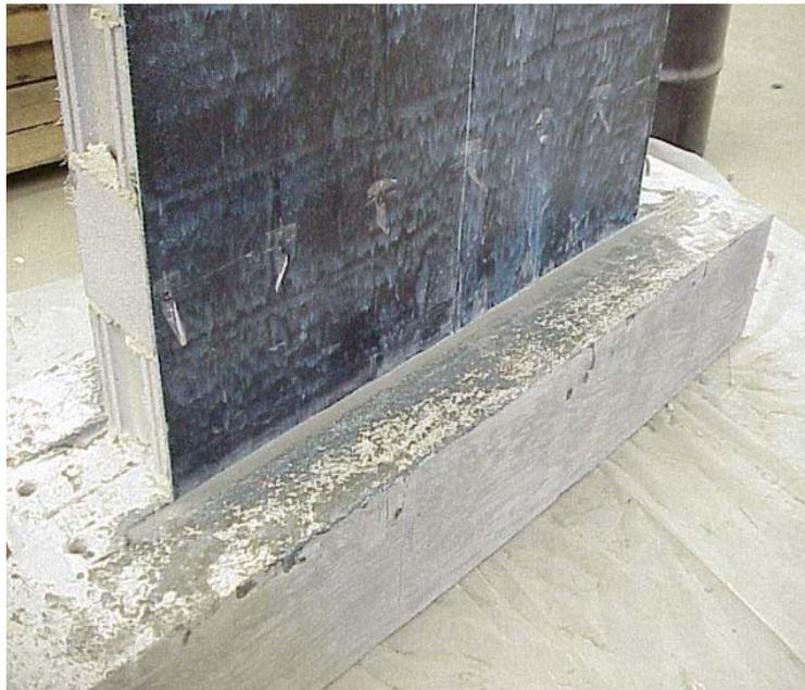
Figure 3. Composite anchor into wall foundation
