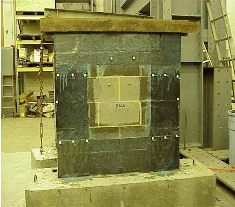
Figure 2. Retrofitted shear wall specimen
