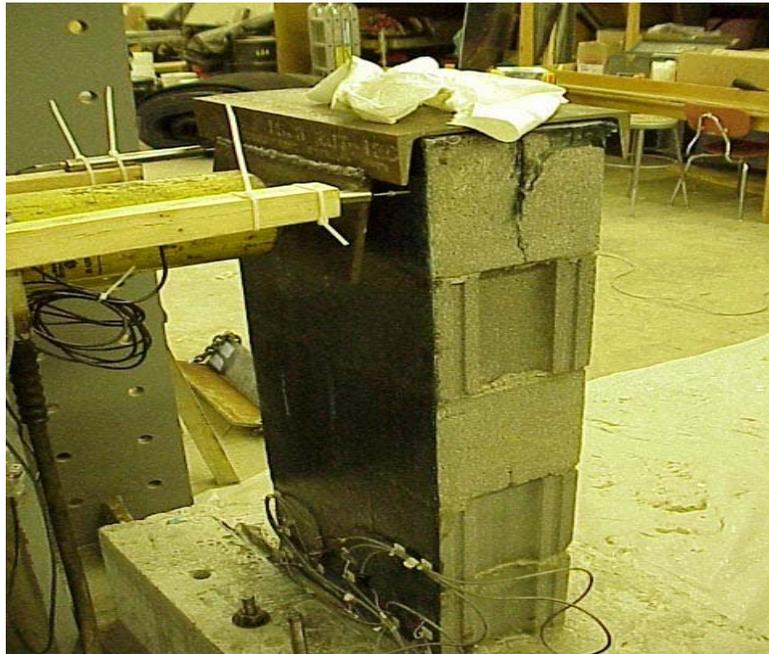
Figure 1. Retrofitted bending wall specimen
