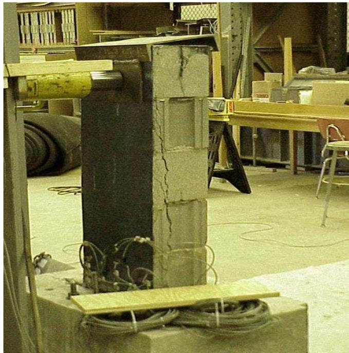
Figure 7. Failure of retrofitted wall subjected to out-of-plane bending
