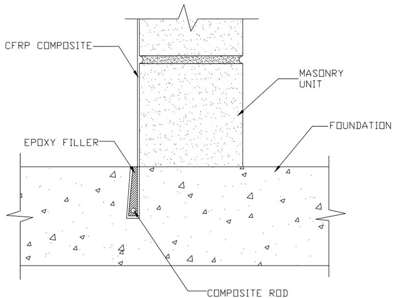
Figure 4. Details of the composite anchor
