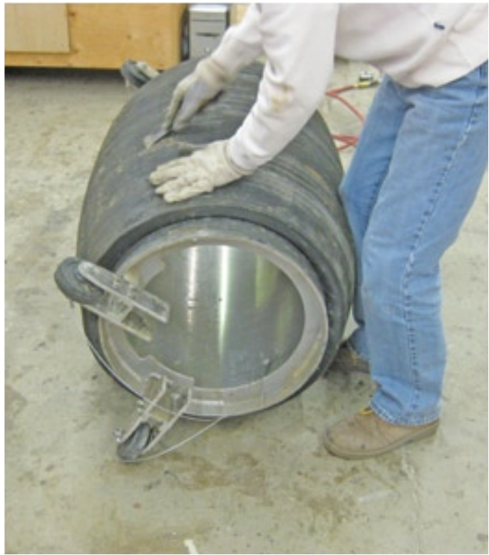
If the diameter of the pipe is small and human entry is not possible, the pipe can be repaired using a packer.
